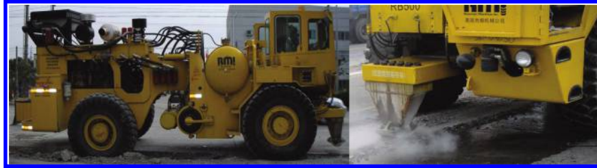
Fig. 2. Resonant frequency breaker used in trial sections.
